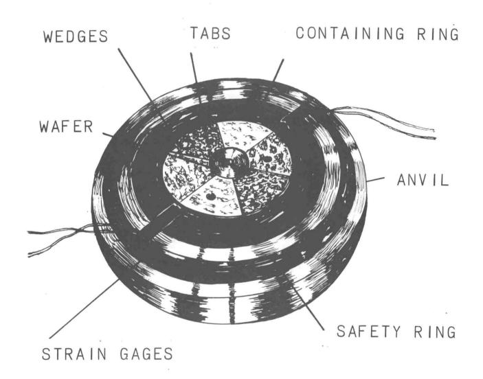
FIG. 4 ASSEMBLY VIEW OF WAFER CONTAINING RING
